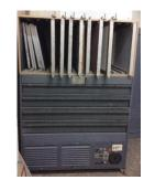
Figure 11, Grand Drying Cabinets, it was designed to be dismantled and reassemble easily for transportation, because of its big size. 100x70cm
