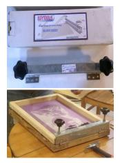
*Figure 27, Using the hinge clamps to produce colored prints and controlling the color effects, on A4 paper. Figure 28, Hinge clamps, designed by the researcher.*
