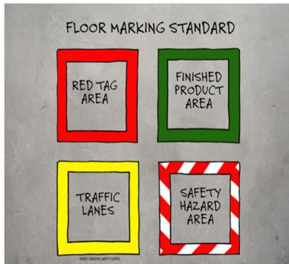
Figure 9, Color coding in industrial projects floor marking
